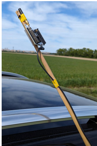
Figure 4.12: Close-up of Nucleo attached to the car acting as the Gateway for range testing.
