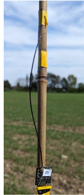
Figure 4.11: Close-up of the pole with Nodes attached for range testing.
