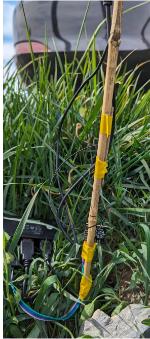
Figure 4.11: Close-up of the pole with Nodes attached for range testing.
