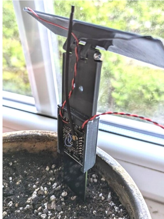
(b) : Close-up picture of the sensor and its housing. The LoRa module is clearly visible, along with the connections to the solar panel, the battery, and the antenna.
