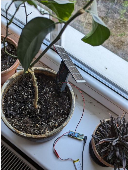
(a) : Soil moisture sensor stuck in the pot (center) on a window sill facing south. The lithium battery is connected externally through the RaspberryPi Pico development board (bottom), acting as a data logger of the voltage and current.
